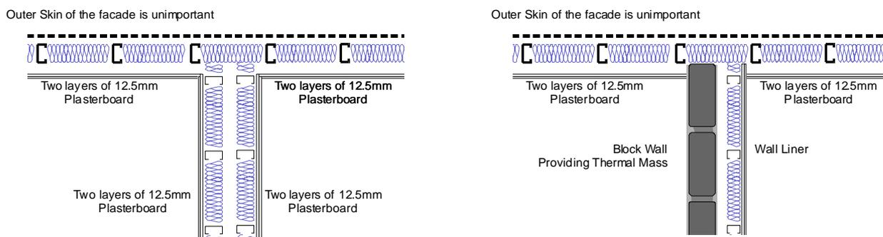
Facade detail – Stud and block work
