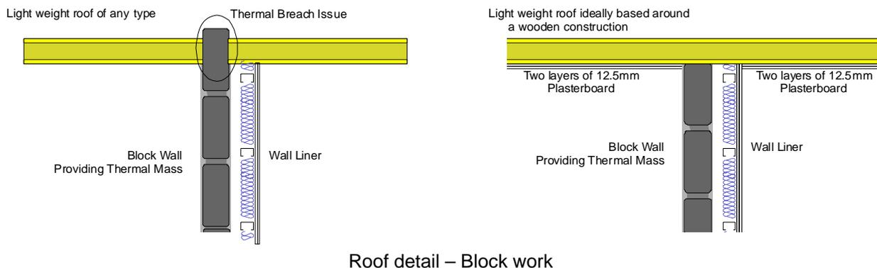
Note, the block wall within the above, right hand side detail, could be replaced with a stud wall.
