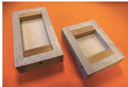
The boxes are provided with a timber strip to allow the installer to screw fix them securely in the cavity. It is advised that a bead of SRS Gripfix adhesive is applied to the edges of the box both to provide a seal and to permanently bond the box to the partition linings.
