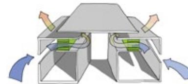
The stack effect, caused by the height difference between the air in-let windows and the air out-let, naturally drives the hot air out of the building. Cowlin Construction, the main contractor, had handed over the project to the University and has therefore asked MACH Acoustics to support the final design and installation of crosstalk attenuators, integrating with existing ducting.
