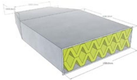
BB93 requires the weighted element-normalized level difference ( $D_{n,e,W}$ ) of 39dB. To achieve this target in the new Graduate School, MACH Acoustics designed 1100mm long NVAs which were installed into bulkheads between the teaching rooms and the main corridor.
